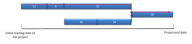
The task durations were classically assessed by each manager in order to obtain, before term, a probability of completion greater than 90%. The diagram highlights the critical path underlined in red.
